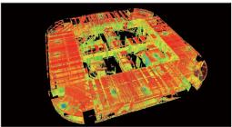
3D scanning data is imported in Autodesk Recap Pro to generate as-build BIM models for interior decoration design and construction guide. It helps the subcontractors to re-optimize their work under the most updated and real conditions, and ensure the completion of project models in as-built status.
